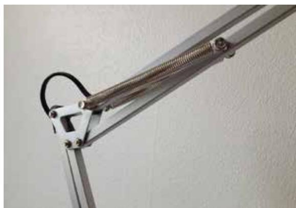
Figure 6: Tension spring of an angle-poise lamp, 2013. Photograph: Kristina Niedderer
